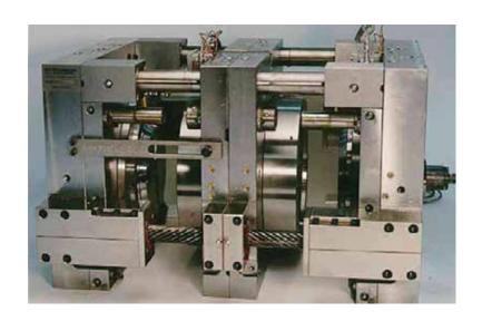
3-Axis High Speed Linear Drive Die Sinker E.D.M
