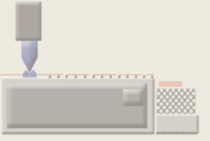
Our cut to length line uses a roll feeding, AC servo drive, with a fully digital length control system that ensures fast positioning.
